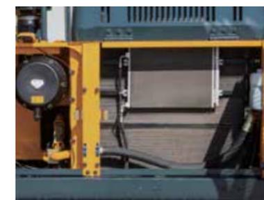
New Cooling System with Increased Air Flow
