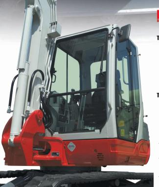
**ISOLATION MOUNTED PLATFORM** minimizes noise and vibration
