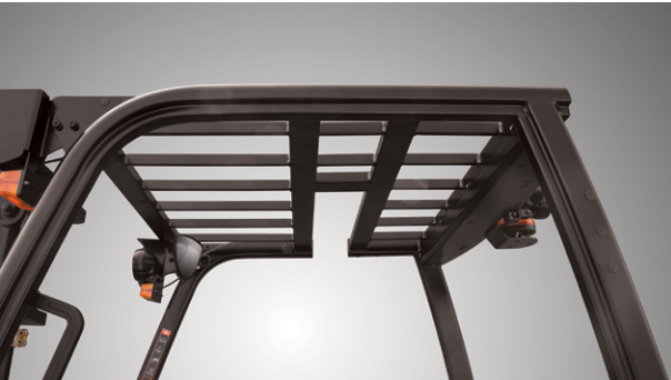
Strong overhead guard Exceeding EEC and ANSI regulations, the overhead guard offers great protection combined with excellent all around visibility.
