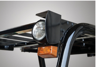
Safety lamps & rear reflectors Halogen headlights and rear LED combination lights offer the driver visibility in all circumstances. Rear reflectors mounted on the counterweight enhance safety for the driver and the application.
