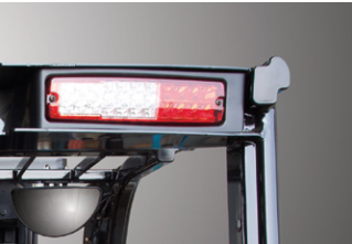
Safety lamps & rear reflectors Halogen headlights and rear LED combination lights offer the driver visibility in all circumstances. Rear reflectors mounted on the counterweight enhance safety for the driver and the application.
